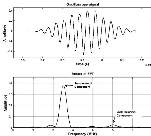
Fig. 3. Typical time-domain signals and frequency spectrum of a surface wave received from an as-solutionized aluminum alloy specimen.
