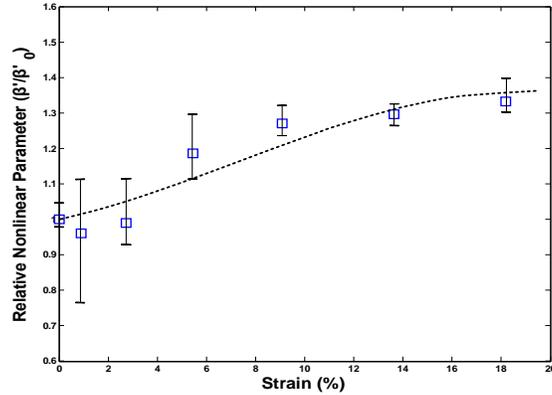
Fig. 4 Relative acoustic nonlinear parameter as a function of the tensile strain.
