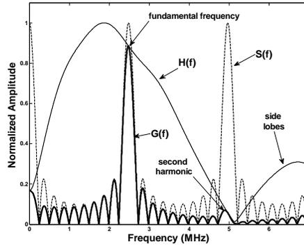
Fig. 1 Theoretical frequency spectra of narrowband surface waves generated by single and multiple line-arrayed rectangular pulse laser beams,  $H(f)$ ,  $S(f)$ ,  $G(f)$ .
