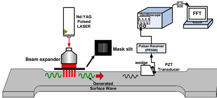
Fig. 2. Schematic diagram of the experimental setup for the measurement of the acoustic nonlinearity of a laser-generated surface wave.
