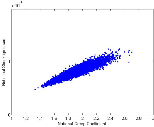
Fig. 2 Statistical dispersion of shrinkage and creep
