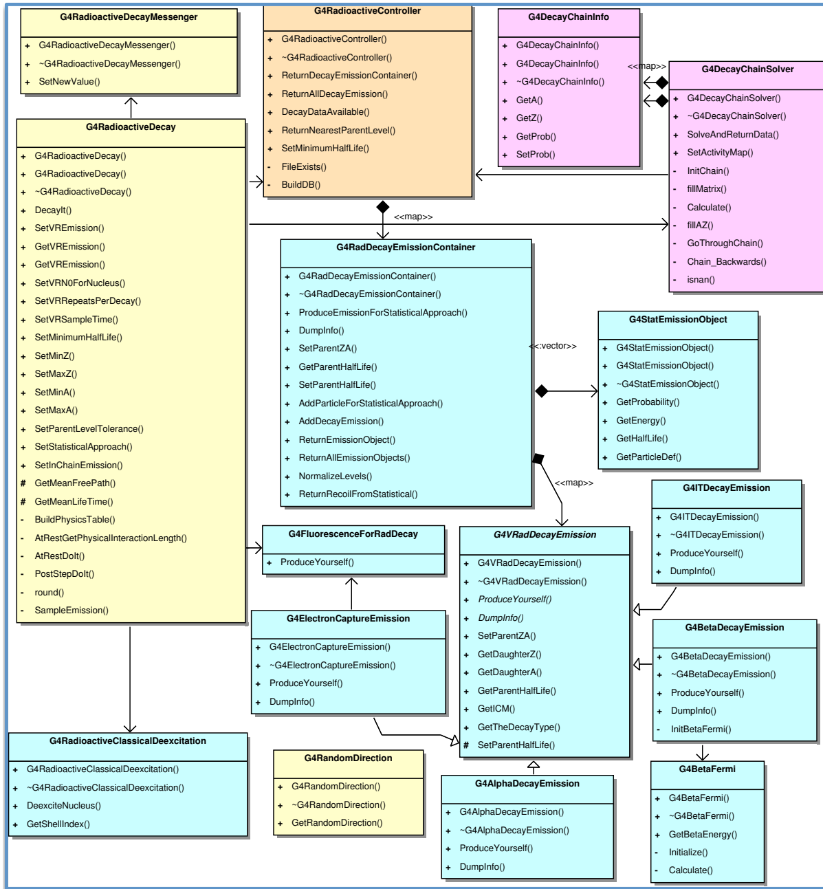
Figure 4. Class diagram of Geant4 radioactive decay resulting from the reengineering process.
