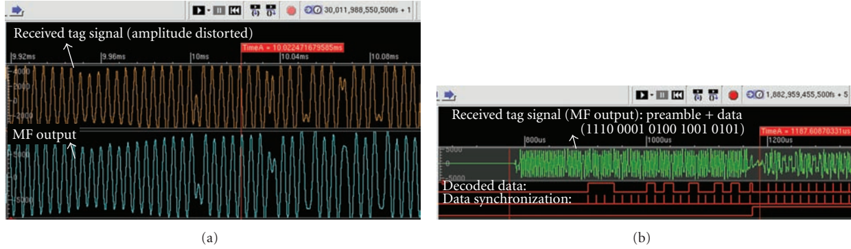
FIGURE 15: FPGA implementation results of the baseband MF demodulator: (a) MF result; (b) symbol detector result.
