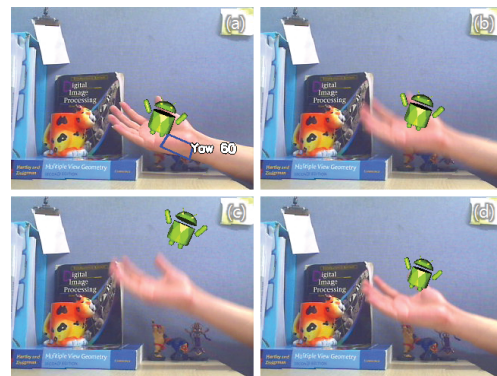
Figure 4. Jump interaction with the android character when the hand is shaking (the procedure is from (a) to (d)).
