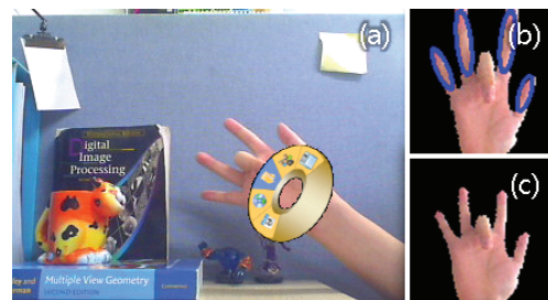
Figure 5. Menu selection using fingers. (a) Menu selection, (b) hand's frontal view and finger gesture recognition, (c) detected hand.
