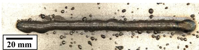
FIG. 4. Bead appearance in GMA-WAAM of the Ti-6Al-4V alloy.
