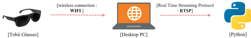
Figure 6: Networking communication structures.
