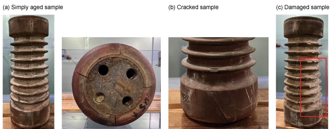
Figure 7. Samples used in the experiment. (a) Simply aged sample; (b) cracked sample; (c) damaged sample.
