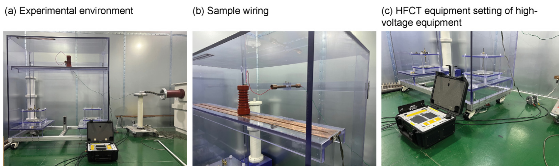
Figure 8. Photographs of the experimental environment. (a) Experimental environment; (b) sample wiring; (c) HFCT equipment setting of high-voltage equipment.
