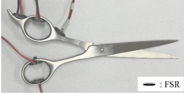
FIGURE 2 The force sensitive resistors are attached to the contact points on the scissor handle.
