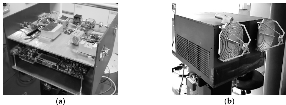
Figure 6. Photographic image of the W-band radar system: (a) interior and (b) exterior.
