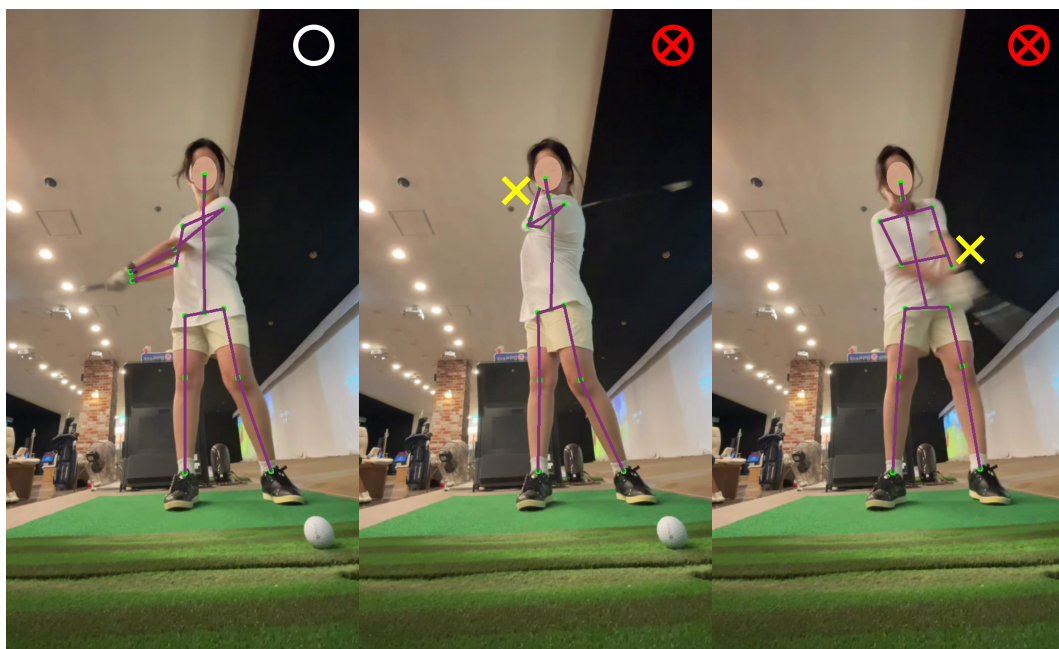
Figure 3. The cases of pose error in the pose estimation process. A white circle indicates that there is no problem with joint coordinate extracted by pose estimation model, and a red symbol means that there is a problem with joint coordinate. A yellow cross sign indicates where the problem occurs. The first image displays a correct or exemplary pose. The second image depicts an incorrect pose due to occlusion. The third image highlights a pose error in the right hand, resulting from image blurring due to rapid motion.
