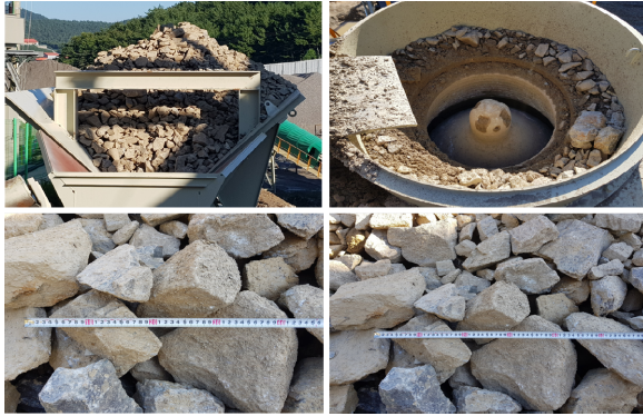
Fig. 5 Rock specimen used for cone crusher vibration test.
