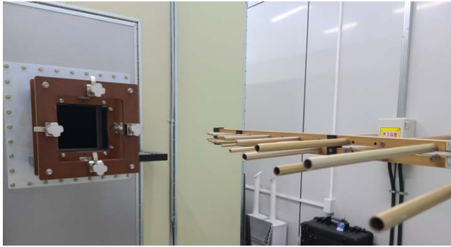
FIGURE 21. Environment for testing the SE of the concrete block.
