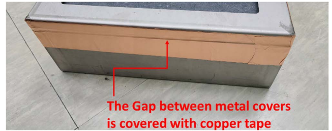
FIGURE 17. Copper tape sealing the gap between the upper and lower metallic covers.
