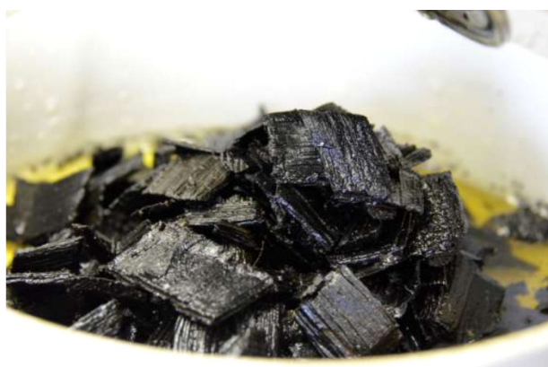
Figure 6. HTP catalyst biofuel from wood chips being separated from the catalyst solution using vacuum filtration.
