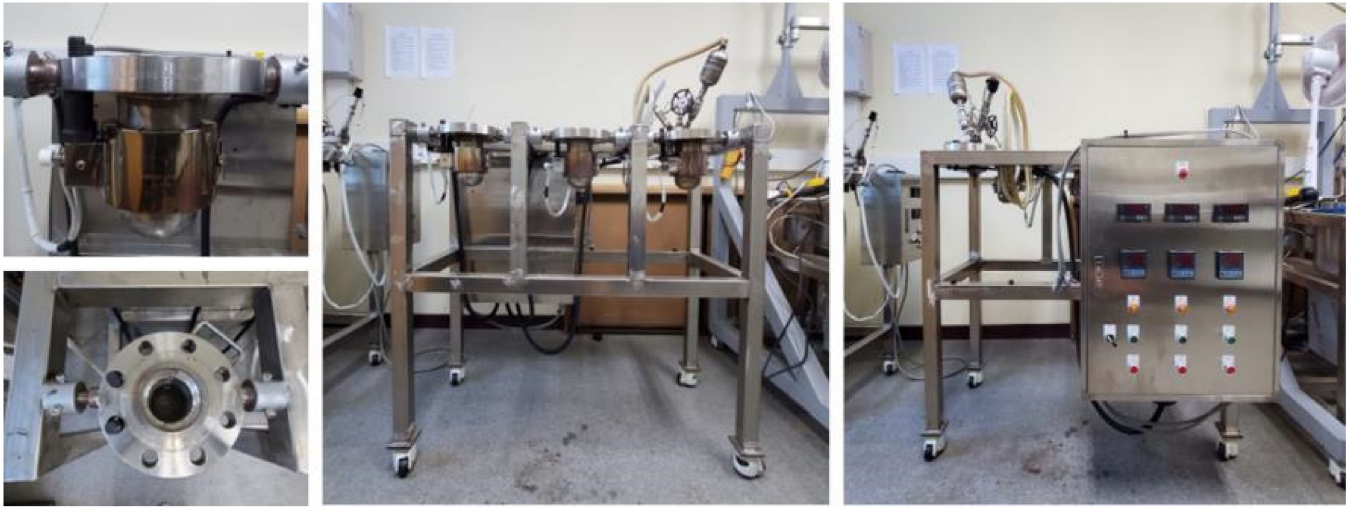
Figure 1. Laboratory-scale hydrothermal carbonization reactor (0.2 L).
