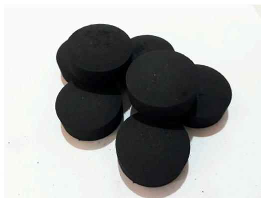
Figure 10. Fabricated combustible briquettes.
