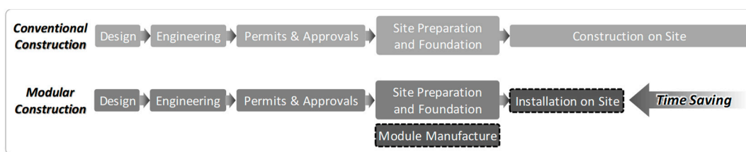
Figure 2. Comparison of modular and conventional RC construction methods, adapted from ref. [11,42].
