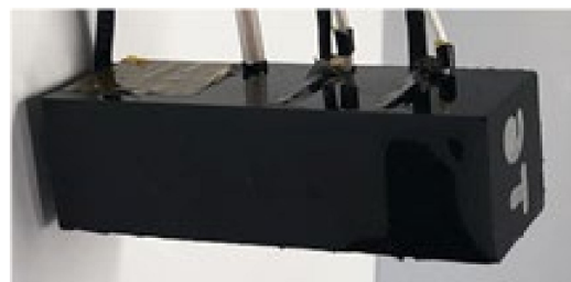
Figure 2. Single smart skin absorber.
