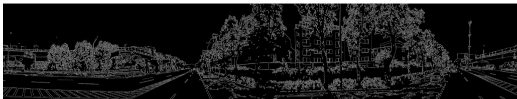
Figure 4. The image from Figure 1 with each object's edges extracted by edge detection.
