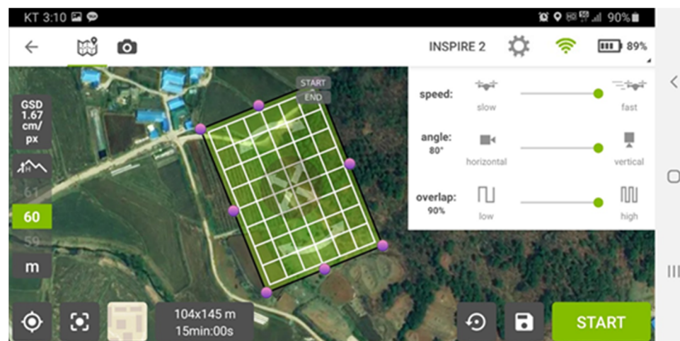
Figure 3. The UAV's flight path setting; a screenshot of the Pix4D app.
