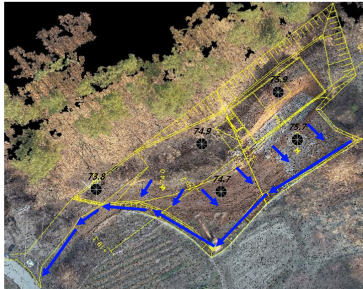
Figure 5. Drainage flow of the site.
