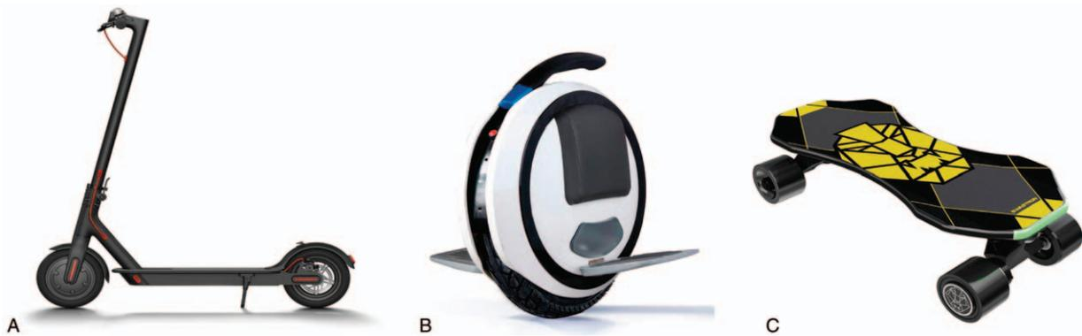
**Figure 1.** Type of personal mobility devices. (A) Electric standing scooter (E-scooter), (B) self-balancing wheel (E-wheel), and (C) electric board (E-board).
