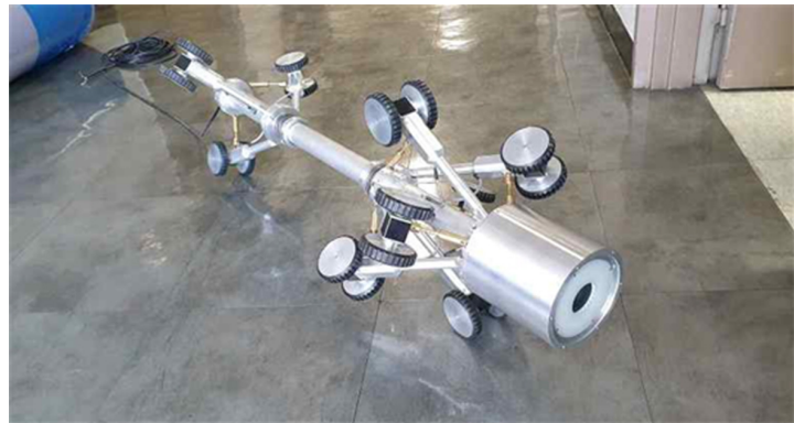
Fig. 3. Borehole alignment tracking and geological exploration system
