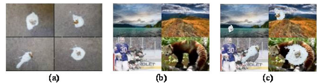
FIGURE 3. Used avian feces data set for training YOLOv3 module. (a) is original artificial avian feces image, (b) is a random background image to be composited, (c) is composited training set image.
