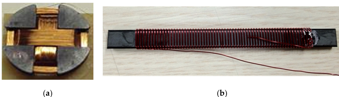
Figure 3. Ferrite antennas used in the automotive field. (a) Keyless entry system; (b) smart key system.
