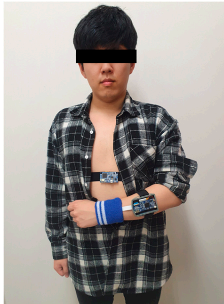
Figure 3. The picture of the subject being equipped with an ECG and multi-channel PPG measurement system.
