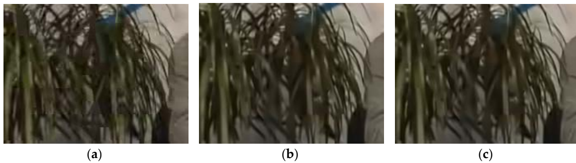
Figure 3. Comparison of the enlarged red box in Figure 2: (a) result for the decoded image using the non-weak filtering method on HM 16.20; (b) result for the decoded image with conventional versatile video coding (VVC) 6.0; (c) result for the decoded image using the non-weak filtering method on VVC 6.0.
