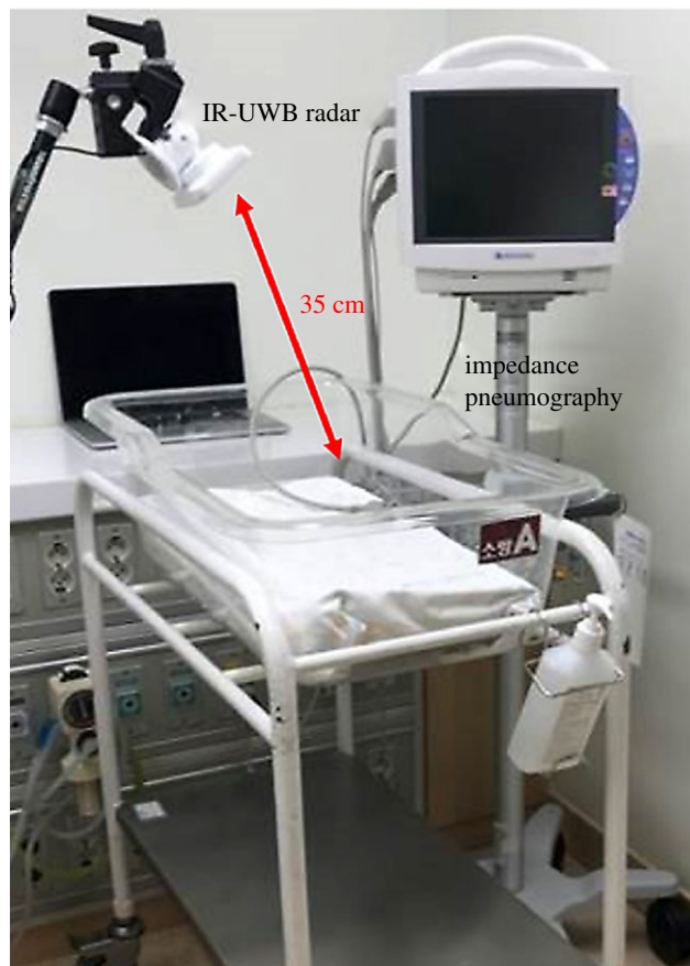
Figure 1. Experimental set-up for simultaneous IR-UWB radar and IP recording. A white cap-covered radar sensor (width \times depth \times height: 5.8 \times 3.4 \times 1.8 cm; weight: 150 g; inside the actual sensor chip: 2.2 \times 1.2 \times 0.6 cm, 18 g) is mounted at the end of a specially designed arm. The BSM-6501 K monitor (Nihon Kohden, Tokyo, Japan) is used as a reference.
