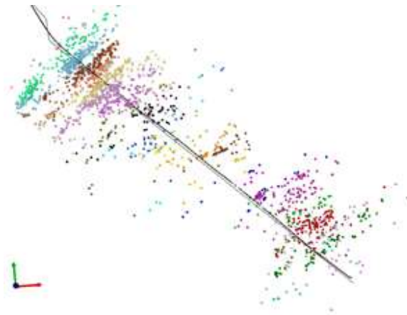
Figure 8. Microseismic signals for the each of stages in target well.
