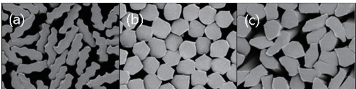
Figure 5. SEM images of cross section according to yarn type (a) 83/36 FD, (b) 100/48 SD, (c) 100/48 DTY.
