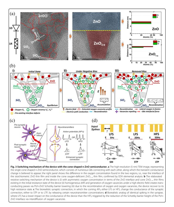
processes of the extended oxygen vacancies profile and previously laterally pushed oxygen will occur. Subsequently, the recovery of the stoichiometric ZnO thin film near the top of the Pt/n-ZnO interface will appear, leading to the back-increased Schottky barrier height and, therefore, the initial resistance state of the device.
