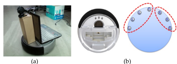
Figure 1. Robot with collision sensor. (a) Two-wheel robot with Web camera, (b) configuration of collision sensors.
