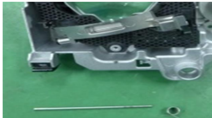
Figure 5. Breakdown of a return-spring in a bi-functional DC motor.
