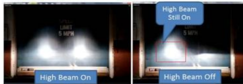
Figure 2. Fault phenomenon of a headlight system.
