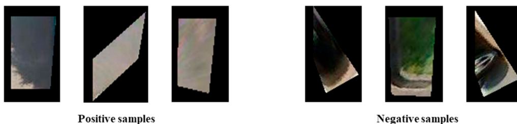
Figure 13. Training samples of vacant parking slot classifier.
