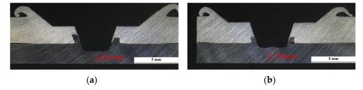
**Figure 11.** Cross-sections of friction stir spot welding (FSSW) for dissimilar metals (**a**) with and (**b**) without control (plunge depth: 4 mm; stirring time: 6 s; tool rotation speed: 1500 rpm; material: Al 6061-T6 alloy (top) and SPFC 590 dual phase (DP) steel (bottom)).
