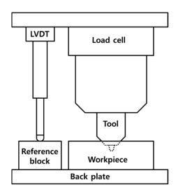
Figure 2. Set-up of the sensing system.
