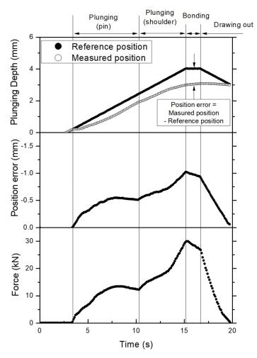
**Figure 3.** Measured profiles of plunge depth, deflection, and force during friction stir spot welding (FSSW) of steel (SS400).
