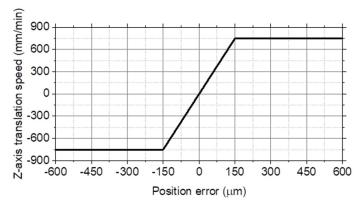
**Figure 7.** *Z*-axis translation speed according to position error.
