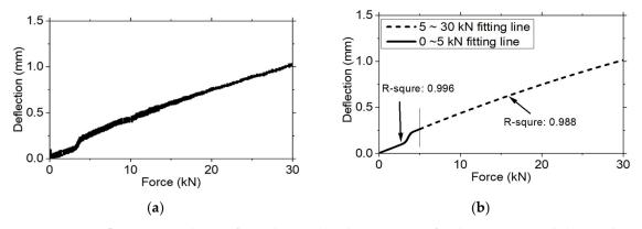
**Figure 4.** Deflection according to force during the plunging stage for the (a) measured data and (b) fitted results.
