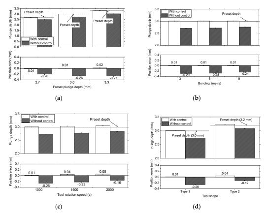
**Figure 9.** Effect of process parameters (parameter details given in Table 1) for (**a**) preset plunge depth (exp. No. 1–3), (**b**) bonding time (exp. No. 4–6), (**c**) tool rotation speed (exp. No. 7–9), and (**d**) tool shape (exp. No. 10 and 11).
