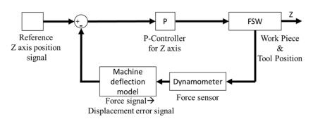
Figure 6. Feedback controller block diagram.
