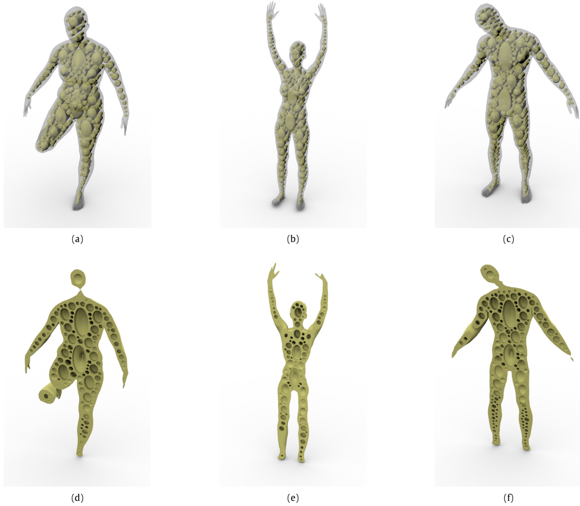
Fig. 10. Hollowed human models with different poses. The upper row shows the hollowed model and the lower row one of the cross sections.
