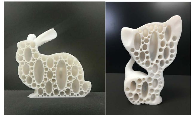
Fig. 12. Photos of the fabricated bunny model and kitten model hollowed by our method.
